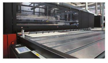
The lamps used for the LED UV curing system contain no Mercury, with low energy consumption and have a life spar of around 10, 000
